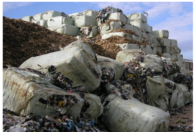
Poor quality recycled material with low value, creating odour and flies nuisance and a fire hazard. Sometimes illegally mis-described as Refuse Derived Fuel.
